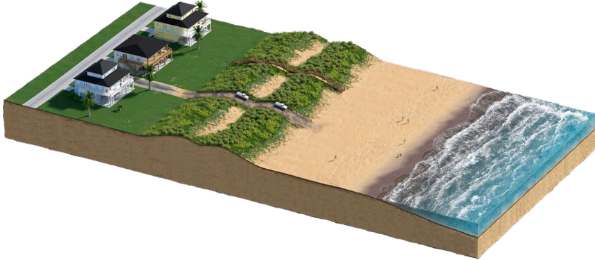
Figure 1: Conceptual rendering of a proposed dual dune beach and dune system with walkovers and driveovers.
